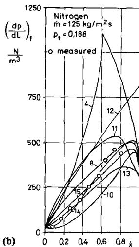
Fig. 5. Influence of flow quality on frictional pressure drop of nitrogen, calculated according to correlations given in Table 1.
