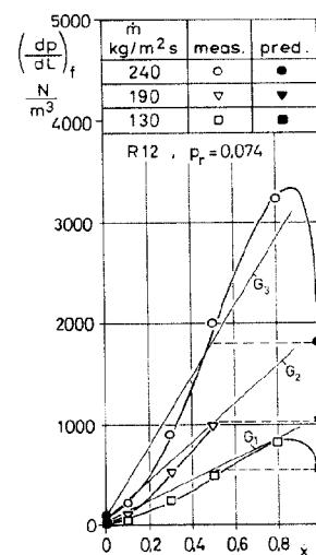
Fig. 1. Influence of flow quality on frictional pressure drop of R12, according to ref. 6.
