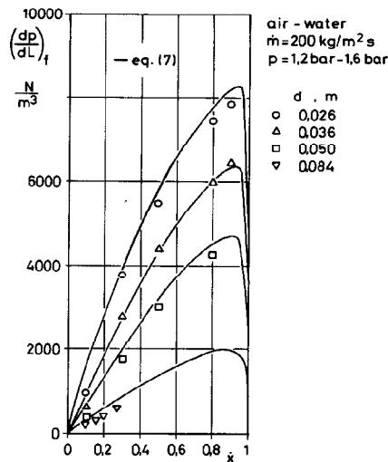
Fig. 2. Measured and calculated frictional pressure drop of water and air as a function of flow quality.
