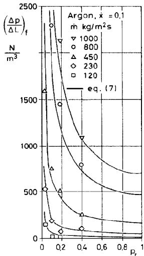
Fig. 4. Measured and calculated frictional pressure drop of argon as a function of reduced pressure.
