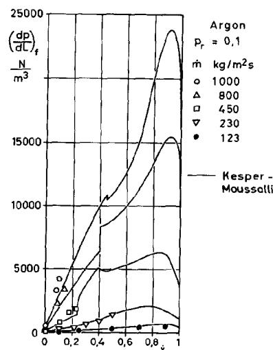
Fig. 6. Frictional pressure drop vs. flow quality, calculated according to ref. 17.
