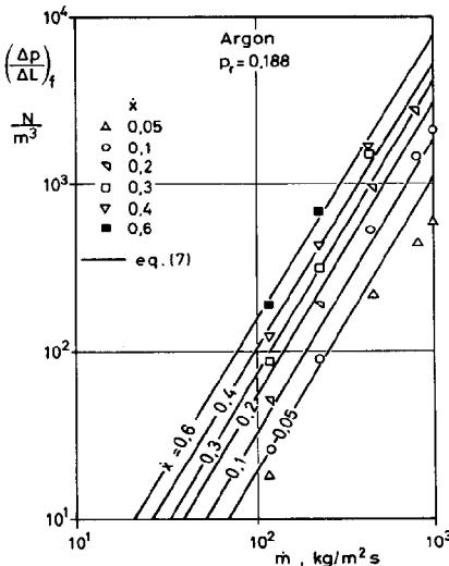
Fig. 3. Measured and calculated frictional pressure drop of argon as a function of mass velocity.
